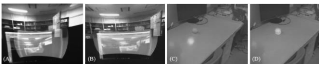
Figure 1: (A) Merged video streams from unsynchronized RGB and thermal cameras attached to a head-mounted display, with registration mismatch resulting from a user's head motion. (B) AR Timewarping applied to streams from A to correct registration. (C) Merged video streams using the same setup as A with registration error resulting from scene motion from the trajectory of a rolling heated ball. (D) AR Timewarping applied to streams from C to correct registration.
